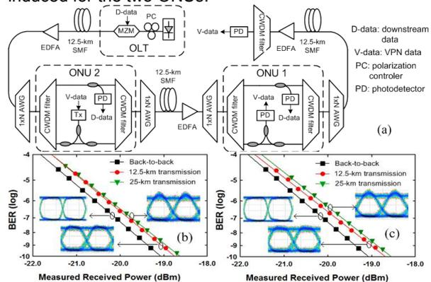
Figure 3: (a) Downstream and VPN experimental setup. BER performances of the 5-Gb/s (b) downstream, and (c) VPN ASK signals.
