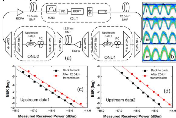
Figure 2: (a) Upstream experimental setup and (b) eye diagrams before and after MZDI. BER performances of the upstream (c) data1 and (d) data2.
